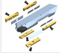
In certain cross drilling operations, the guide pads of the guide part can be fitted with thicker adjusting shims in order to achieve a tighter guidance. The feed rates have to be reduced accordingly.
