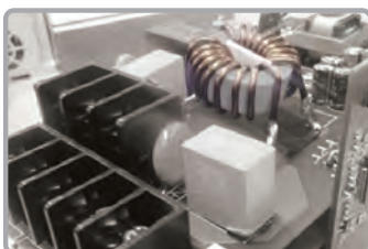
Built-in EMC Filter (C2 class)
